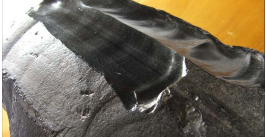
See the difference between the slick, glassy surface of a new break, compared to the dull appearance of the surface of obsidian long exposed to weather, rain, freezing, etc.
